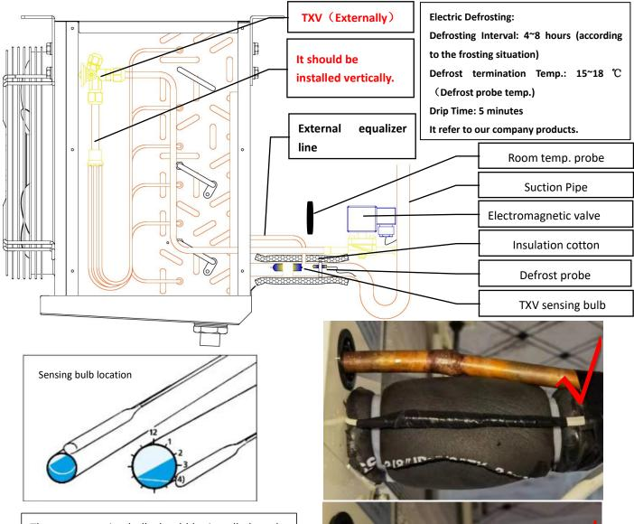
The temp. sensing bulb should be installed on the horizontal suction pipe, and the position should be at 1 o'clock and 4 o'clock position. Position depends on tubing OD.
